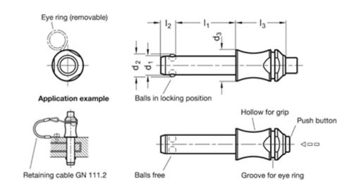
d1 -0.04/-0.08 = - d2 = - d3 = - l3 = - l1 +0.6 = -  $l2 \pm 1 = -$ Load in (N) = Weight in (g) = -
